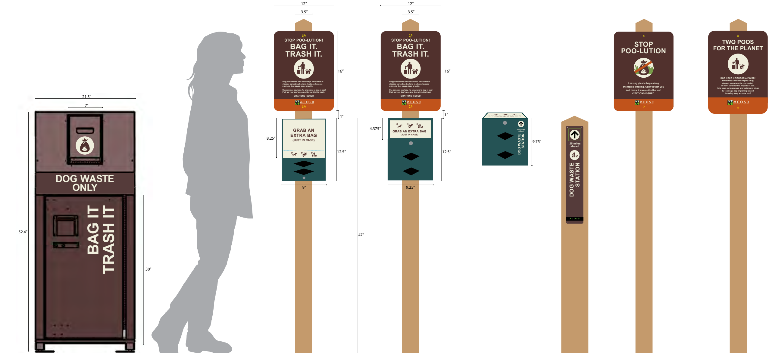
Door Decal 4" diameter Dog Waste Only Decal 12.4" x 3.4" – 1.5" tall letters (150 pt) Bag It Trash It Decal 12.4" x 6.1" – 2" tall letters (194pt)
