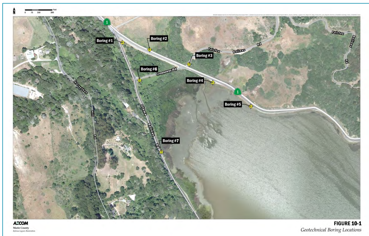
Figure 5: Geotechnical Borings Site Plan
